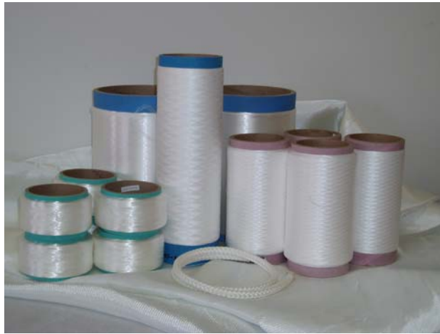
Figure 5. Cyclic olefin copolymer yarns, shown on green and large blue bobbins. The other yarn in the photo is Innegra S, a high modulus polypropylene fiber.
